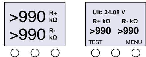
Pressing **TEST** push-button activates test of the device, pressing **MENU** push-button displays the parameters setting menu. Prolonged pressing the middle push-button displays **R+** and **R-** values back again without menu. The signalling relay status is indicated by the symbol of contact. If signalling relay is released (there is no fault in the monitored power supply system), the open contact is displayed. If there is a **FAULT** signalled, the close contact is displayed.
