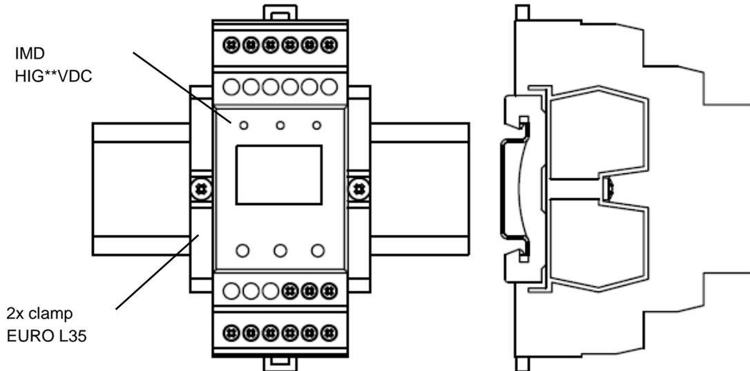
Picture 10: Device assembly in railway applications
