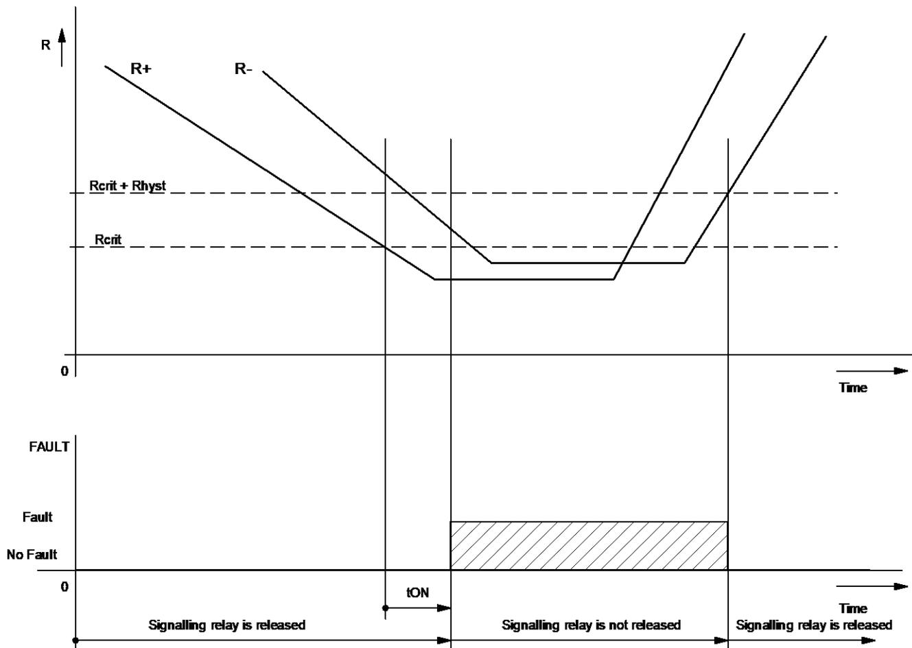
Picture 7: Insulation resistance fault evaluation
